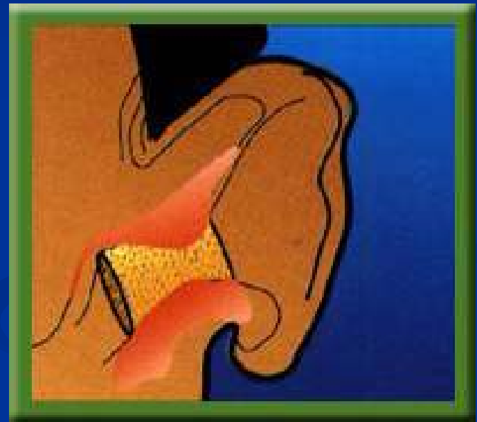
Earplug correctly inserted
