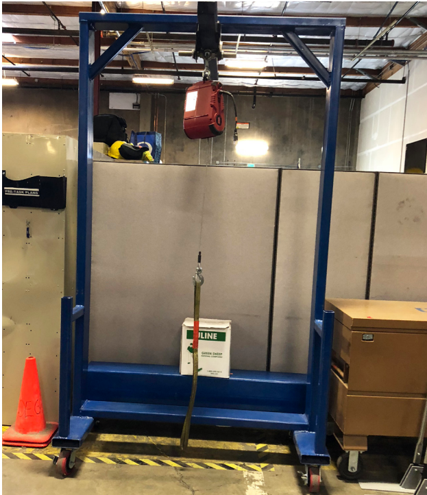
Fig. 3.3: Customized lifter for moving racks of conduit when loading and unloading
